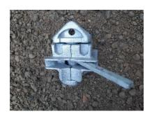
**Transverse Double Ended Twist Lock** The transverse double ended twist lock allows the stacking of containers at 90° to each other.
