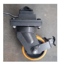
**5 Tonne Container Castor Wheel** Allows you to easily move a container on flat surfaces. Connects directly to the bottom corners of your container. Each has a 5 tonne WLL so giving a combined 20 tonne WLL when using one in each corner.
