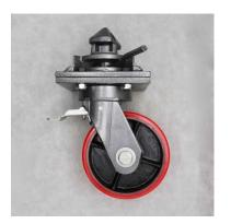
**3 Tonne Container Castor Wheel** Allows you to easily move a container on flat surfaces. Connects directly to the bottom corners of your container. Each has a 3 tonne WLL so giving a combined 12 tonne WLL when using one in each corner.
